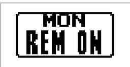
Used for automated households. The remote signal is a potential free contact. The sauna heater switches on when contact is closed and remains on until contact is opened.
