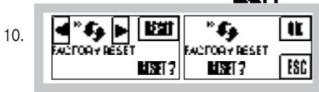
Reset all settings back to factory settings by pressing reset button. Confirm resetting by pressing OK button. Restoring factory settings wont reset kWh and ON hours counters.
