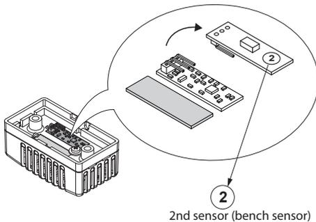
Pin-type connectors in sensor
