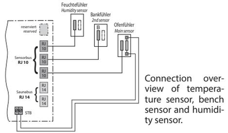
Connection overview of temperature sensor, bench sensor and humidity sensor.
