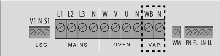
ⓘ The switching output of the control unit for the vaporiser has a max. of 3 kW resistive load. It can be expanded, as needed, by an optional power extension unit (LSG).
