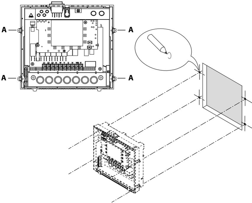
**A** Tabs with mounting holes for screws
