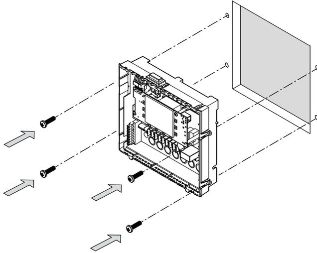
ⓘ You can connect the lines after mounting the housing. See 4 Electrical installation, [EN-38](#).
