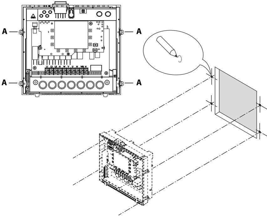
**A** Tabs with mounting holes for screws
