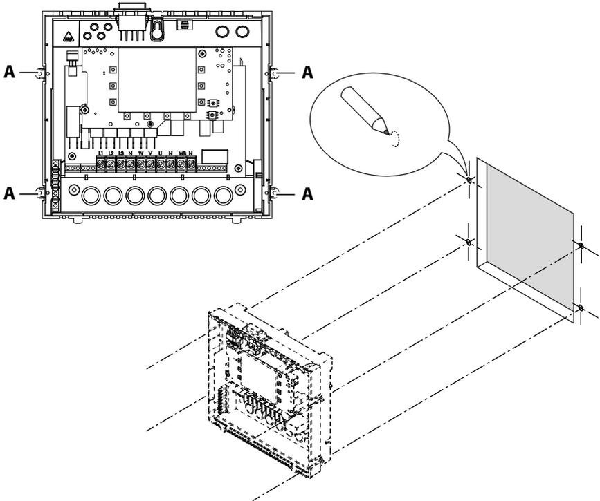
**A** Tabs with mounting holes for screws
