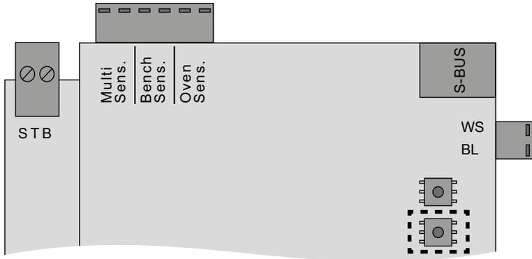
ⓘ Set the jog dial with the screwdriver as supplied in the scope of delivery.
