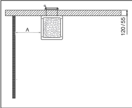
The dimension A is determined based on the safety method used for wooden surfaces.
